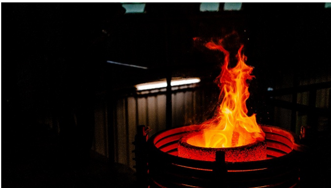
CNMC Photo: Induction furnace at Sokor Gold Project heating up to about 1250 degree Celsius transforming gold mud into gold doré bars
