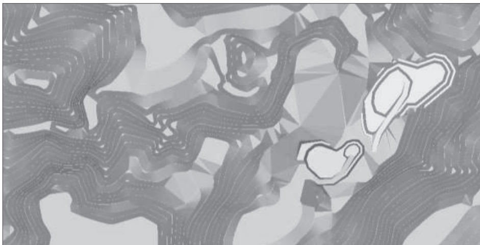
Figure 8.3 Final pit design - Manson's Lode
